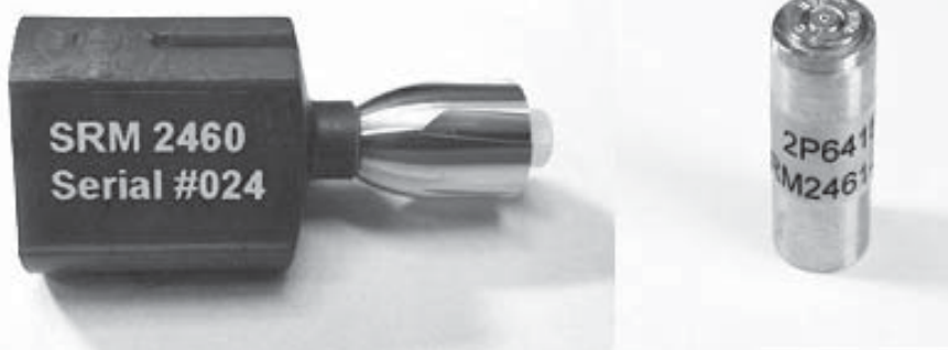
Fig. 1. A NIST Standard Reference Material (SRM) 2460 Standard Bullet (left) and a SRM 2461 Standard Cartridge Case (right)
